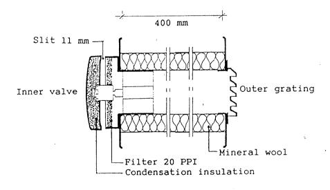
Horizontal section of outdoor air intake. Scale 1:5.
