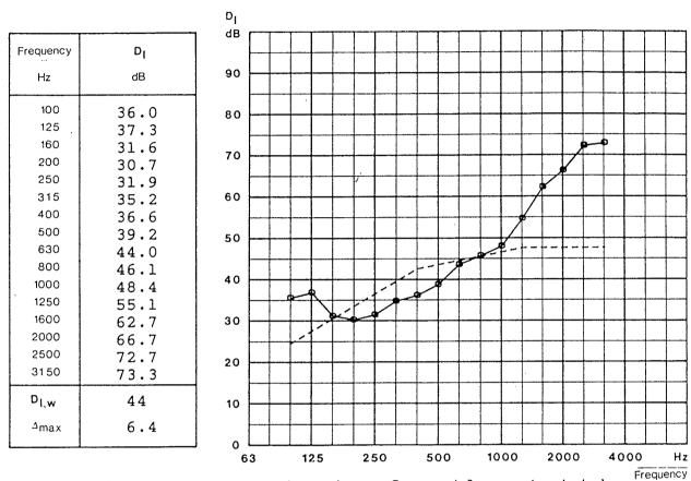
Unit insulation,  $D_{\rm I}$ , per 1/3 octave for outdoor air intake type Fresh 80-dB mounted in a 400 mm wall. The  $D_{\rm I,w}$  reference curve is shown as a dotted line.
