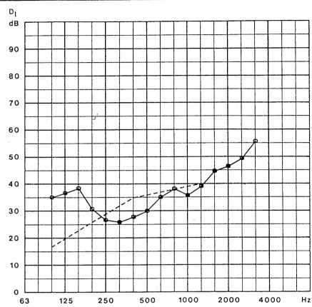
Frequency Unit insulation,  $D_{\text{I}}$ , per 1/3 octave for outdoor air intake type Fresh 80-dB mounted in a 200 mm wall. The DI.w reference curve is shown as a dotted line.
